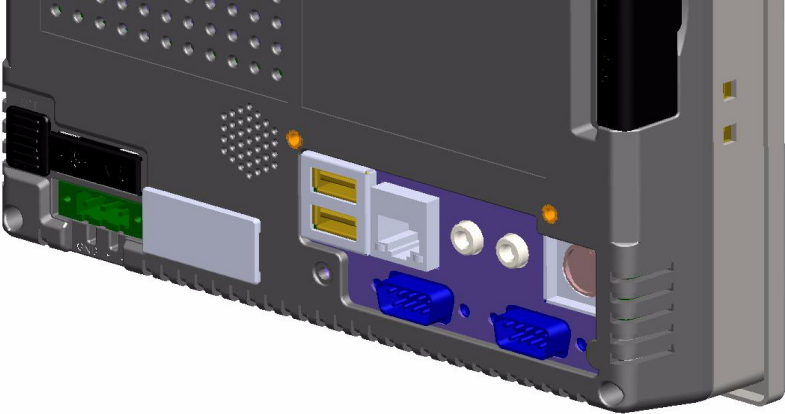
Figure 1.1: I/O Port Arrangement
